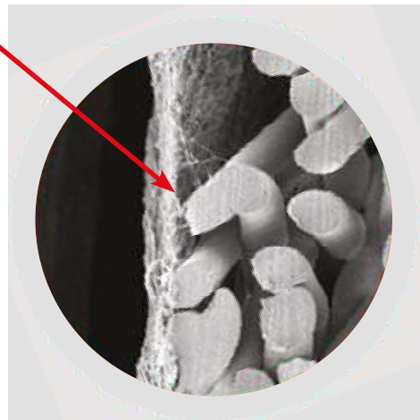
PTFE membrane. Even smallest particles of dust stay on the surface of the material.
